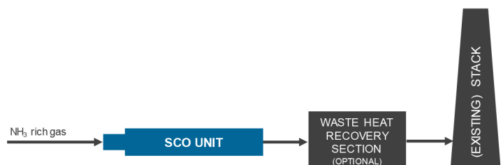
Figure 2 – PFD of basic SCO unit implementation
